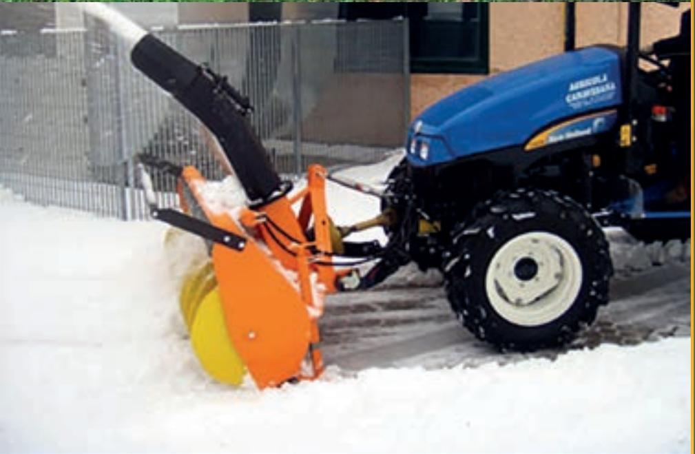
The LS J20 Series Tractors can be fitted with a “CAT 0” Linkage. Attachments can be powered by a front PTO kit.
